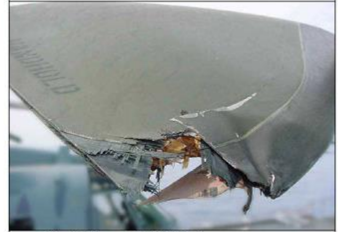
Tip Strike on AW101 Blade (Crown Copyright)
